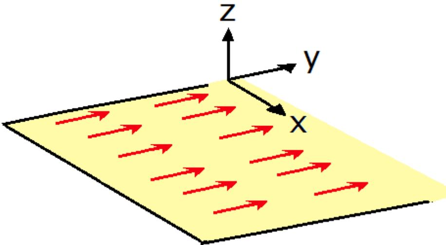
Sheet of current (the direction of current is in +y direction)
