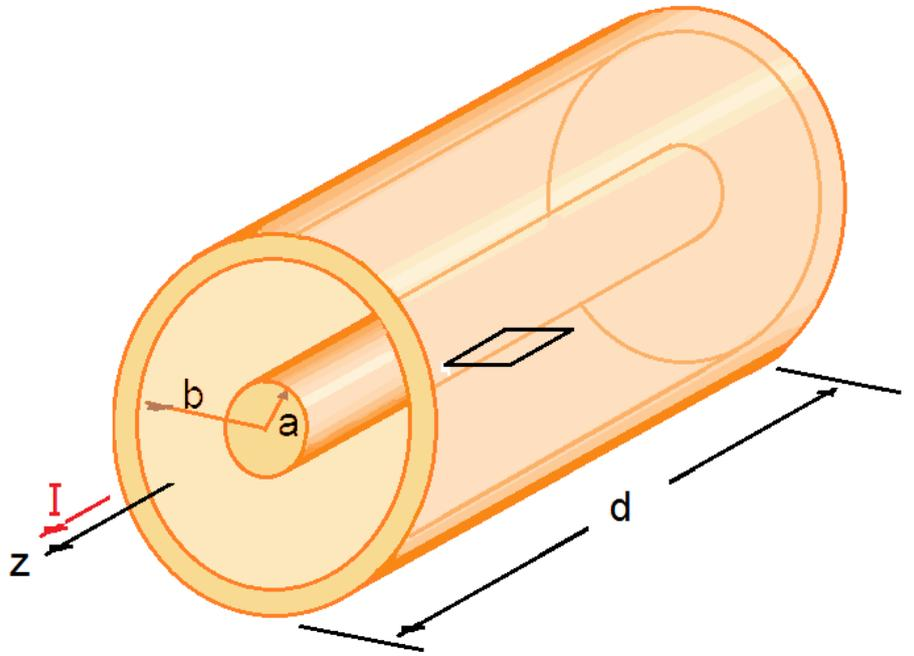
**Exercise:** ( الملزمة ص 111 ) A solid conductor of circular cross section, if the radius  $a=1\text{mm}$ , the conductor axis lies on the  $z$  axis, and the total current in the  $az$  direction is  $20\text{A}$ , find:
