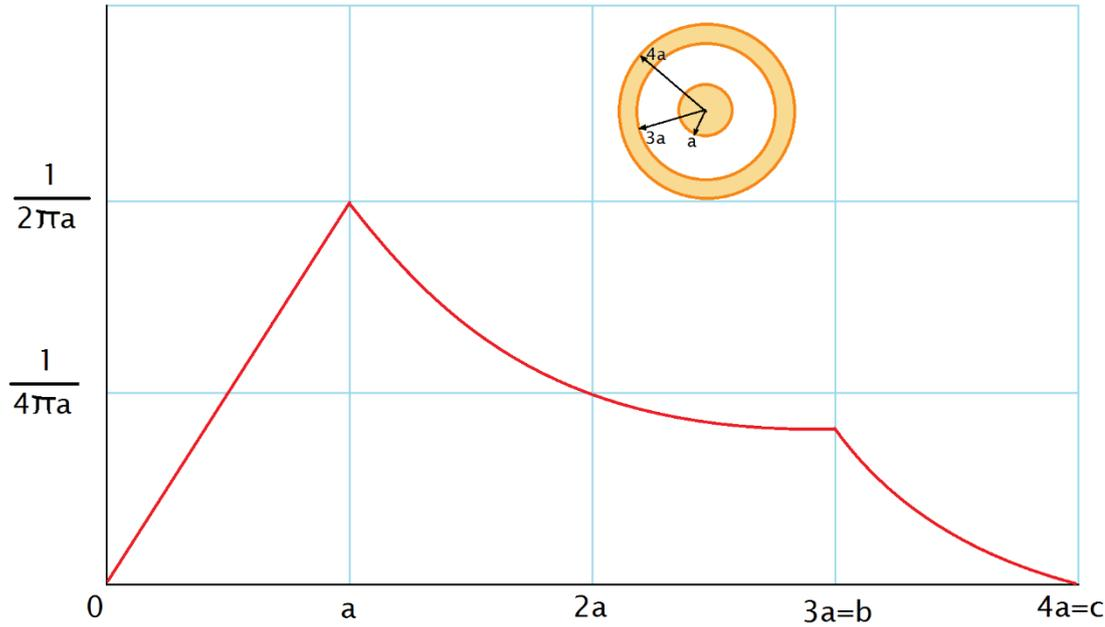
Figure The magnetic field intensity as a function of radius in an infinitely long coaxial transmission line with the dimensions shown.
