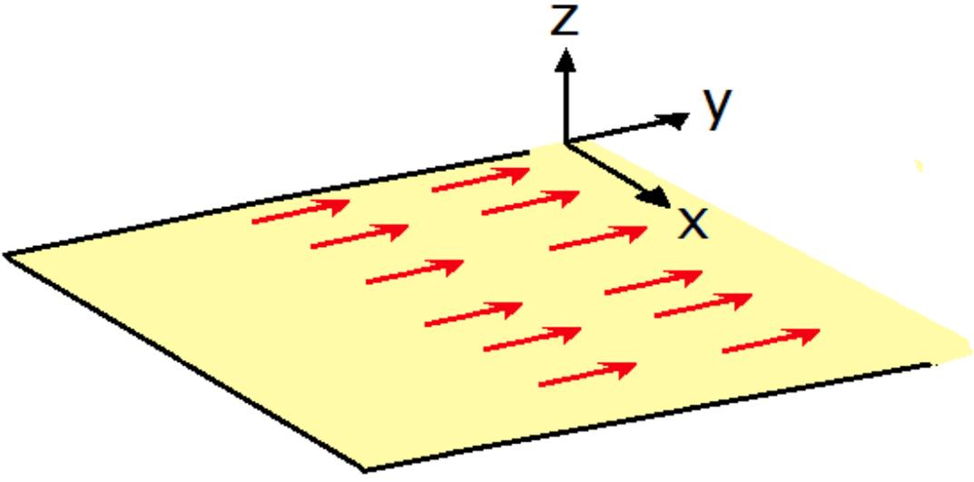
Let ( $\mathbf{a}_N$ ) be a unit vector normal (outward) to the sheet as shown in figure below:
