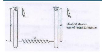
**Q15:** The potential energy of the system shown in Figure at an arbitrary instant  $\theta_1$  and  $\theta_2$  is:
