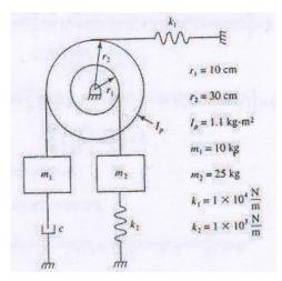
**Q12:** If  $\theta$  and  $\dot{\theta}$  are counterclockwise angular displacement and angular velocity of the disk in Figure. Then the kinetic energy of the system is:
